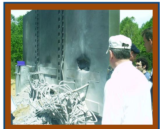
*Image 2 - Damage to concrete bolsters*
